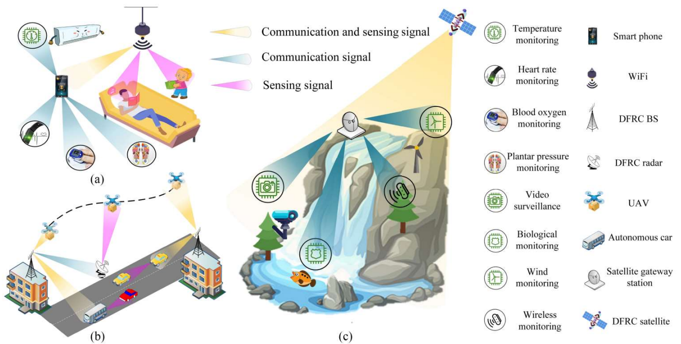
Figure 6.1: Beamforming illustration on three typical JCAS applications: a) smart home, b) autonomous driving, and c) delivery and environmental monitoring
